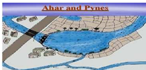
Fig.2- Ahar Pyne system of Bihar
